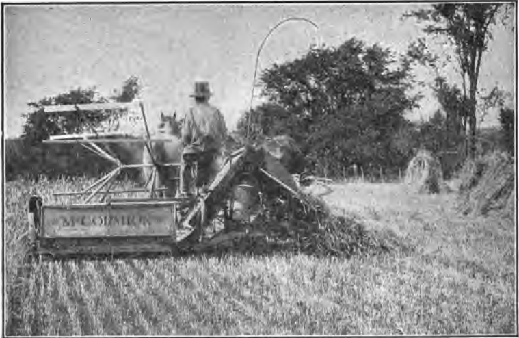
FIG. 16.—Harvesting by machinery in the United States. The machine cuts, binds, and carries the sheaves of small grain. (International Harvester Co.)
